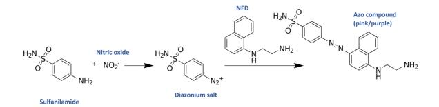
Reagents: 1% Orthophosphoric acid Sulfanilamide Sodium nitrite N-(1-Naphthyl)ethylene diamine dihydrochloride ACS (NED)
